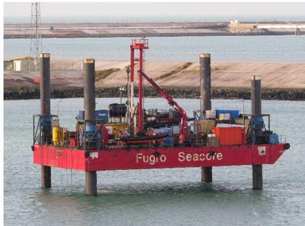
Jack-up Barge Aran 250
